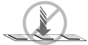
Do not put excessive pressure on surface of tape light (e.g. glass/acrylic panes etc.).
