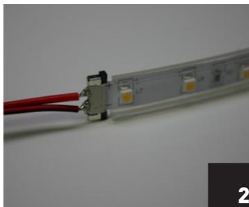
Carefully pull SlimFlex out of silicon sleeve, slide clip connector on (white face up), and slide black portion back towards housing.
