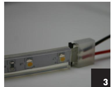
Slide on a provided end cap with holes slide down over wires and fill void with provided silicon glue. Allow 24 hours to fully cure.
